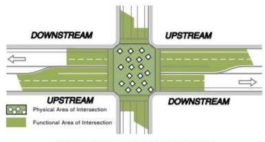
Figure 1: Functional and Physical Areas of an Intersection
